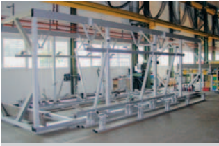
Rail carriage assembly frame
